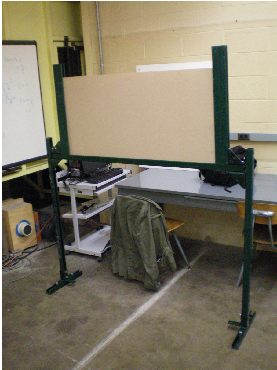
Figure 18: Plexiglas shield and frame for the un-hooded test stand
